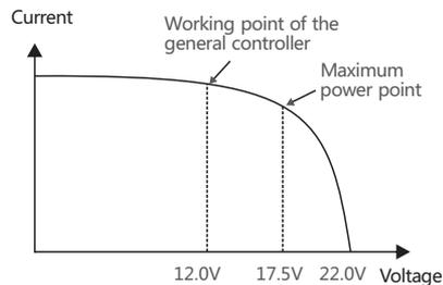
As a charging stage, MPPT can't be used alone. It must be combined with ascending charge, floating charge, equalizing charge to complete the battery charge.
